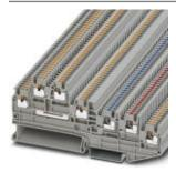
Sensor/actuator terminal block, nom. voltage: 250 V, nominal current: 13.5 A, connection method: Push-in connection, number of connections: 5, cross section: 0.14 mm² - 1.5 mm², AWG: 26 - 14, width: 3.5 mm, height: 44.6 mm, color: gray, mounting type: NS 35/7,5, NS 35/15
